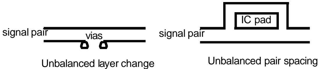
**Figure 33: Avoid Unbalanced Layer Change**
