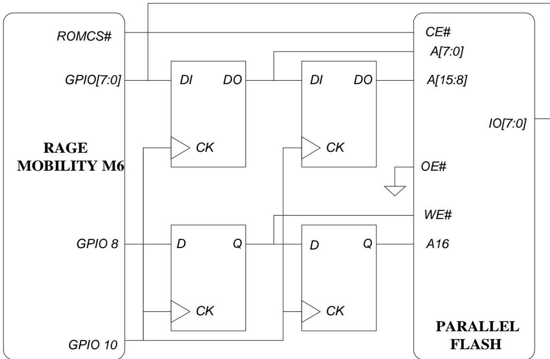
**Figure 28: BIOS Interface – Parallel EEPROM Configuration**
