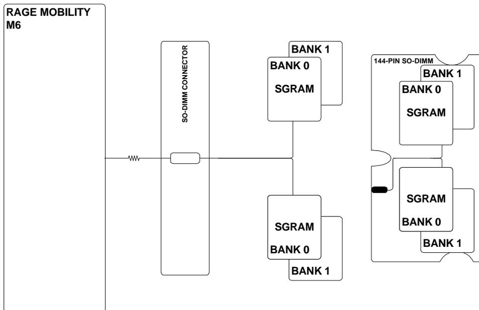
**Figure 21: Address and Control Routing**
