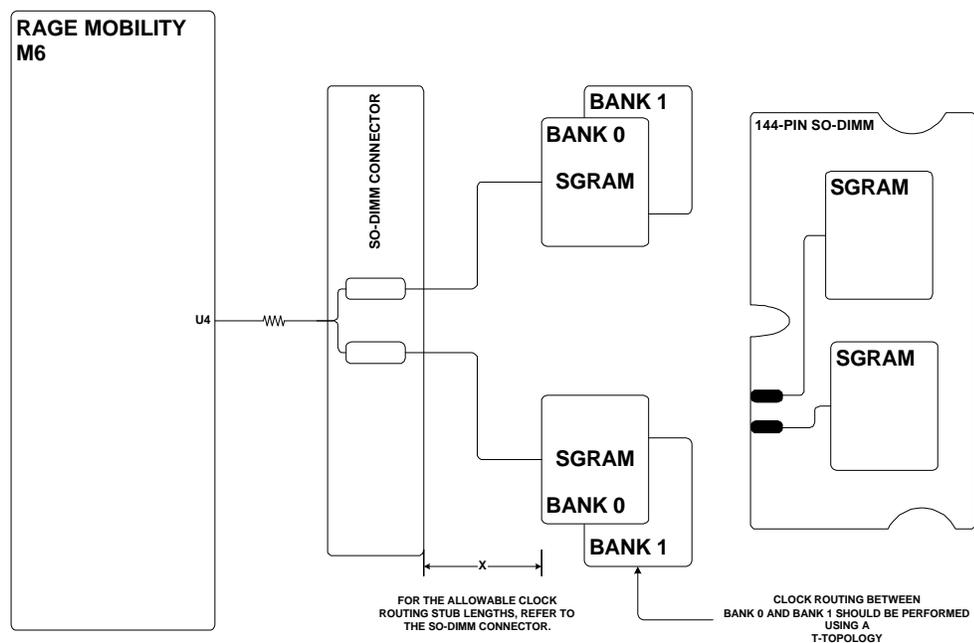
**Figure 19: Memory Clock Routing**
