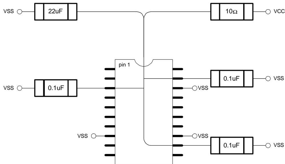
**Figure 41: SM530 Single Power Plane Layout**
