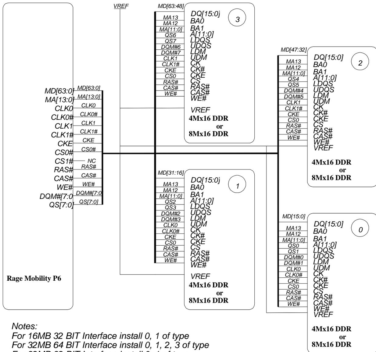
**Figure 14 DDR SDRAM Configuration**
