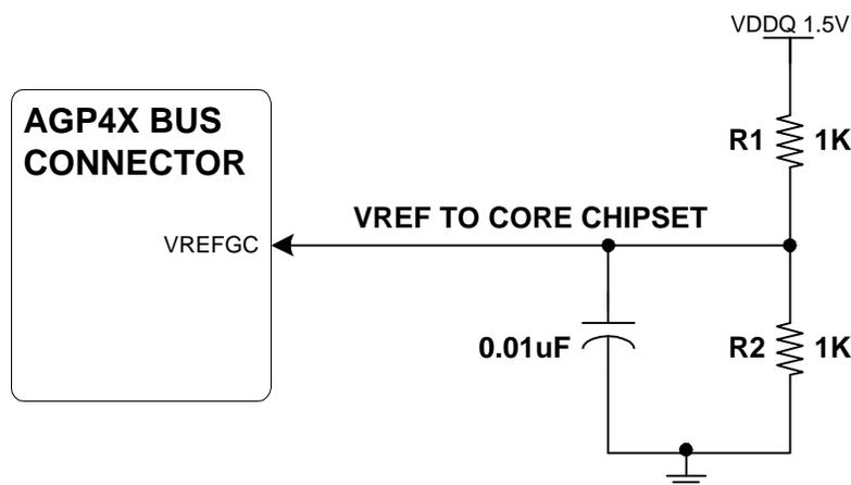
**Figure 6: VREF Voltage Divider Circuit**
