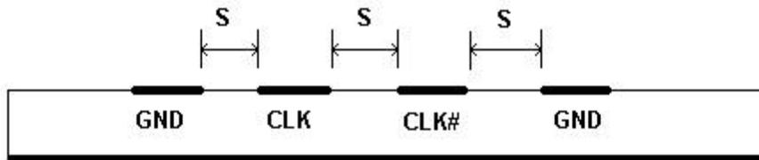
**Figure 22: Clock pair shielding**
