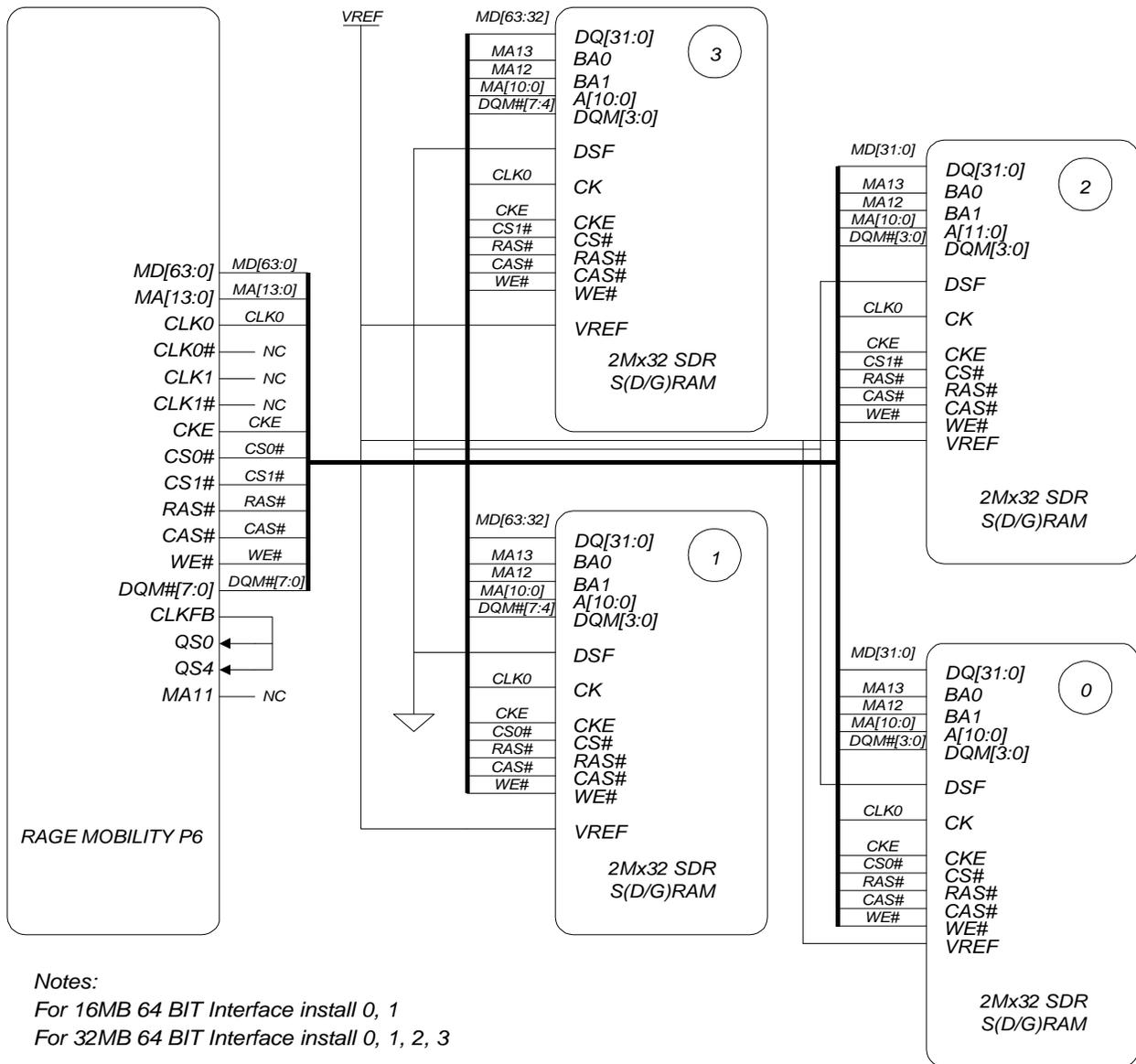
**Figure 16: SDR S(D/G)RAM configuration**
