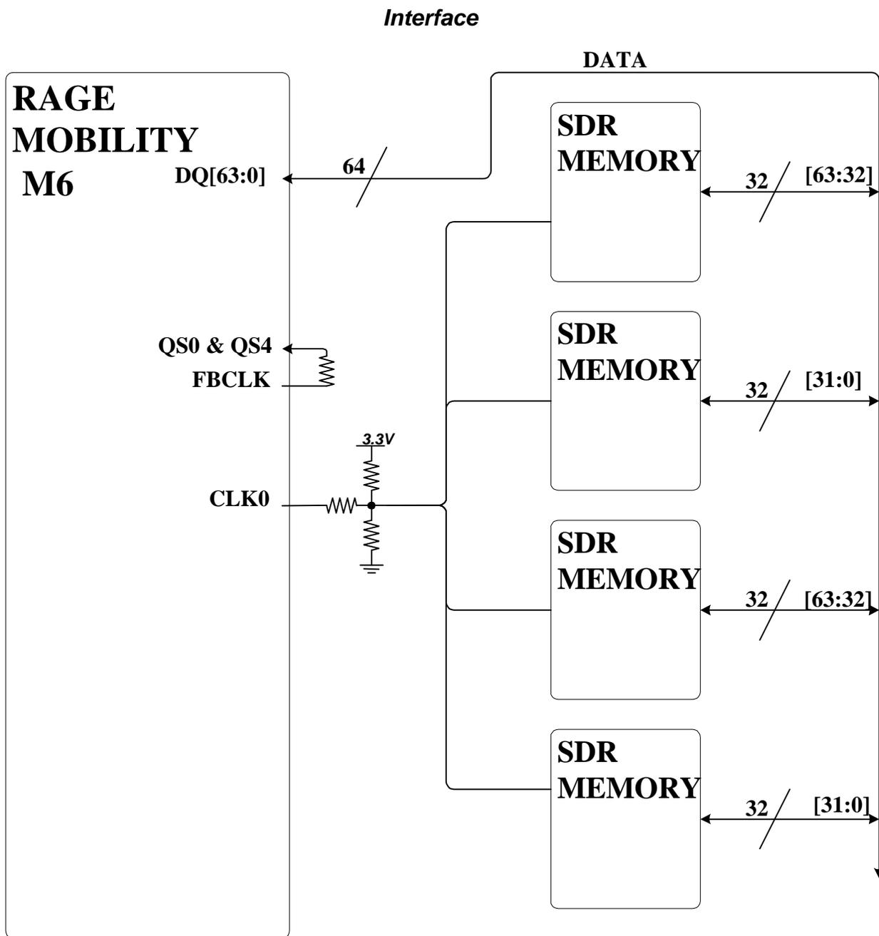
**Figure 18: Memory Clock: Termination and Distribution for the 64-Bit SDR Interface**
