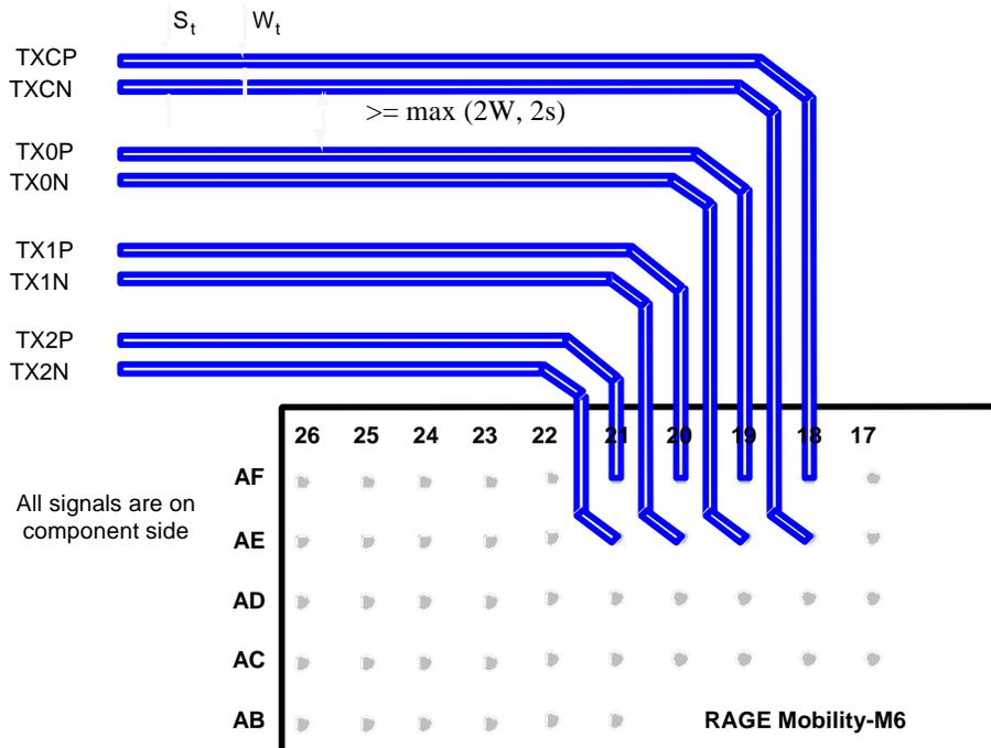
**Figure 32: Routing TMDS Lines**
