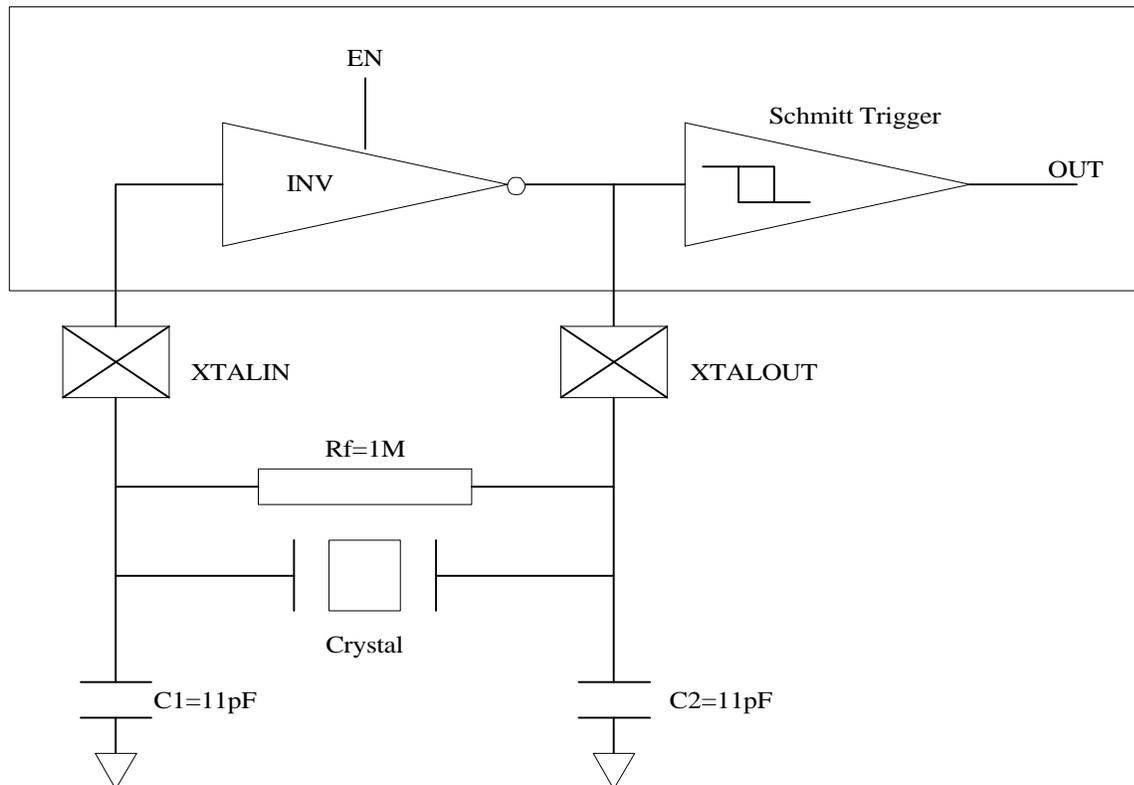
**Figure 30: Oscillator Circuit**
