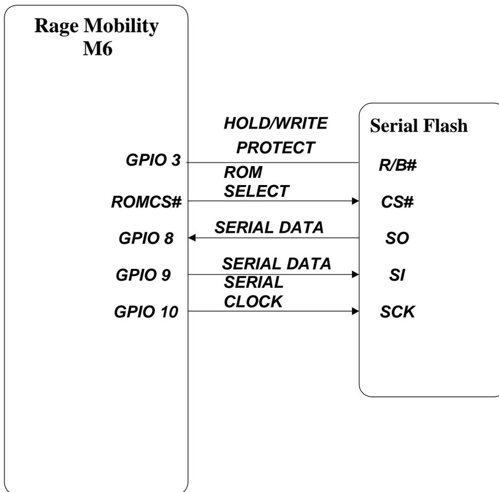
**Figure 27: BIOS Interface – Serial EEPROM Configuration**
