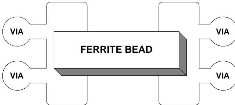
**Figure 2: Typical Installation for a Ferrite Bead**
