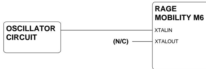
**Figure 10: RAGE MOBILITY M6 with Oscillator**
