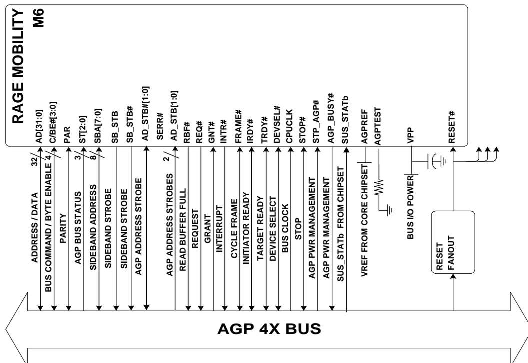
Figure 5: AGP Interface Block Diagram
