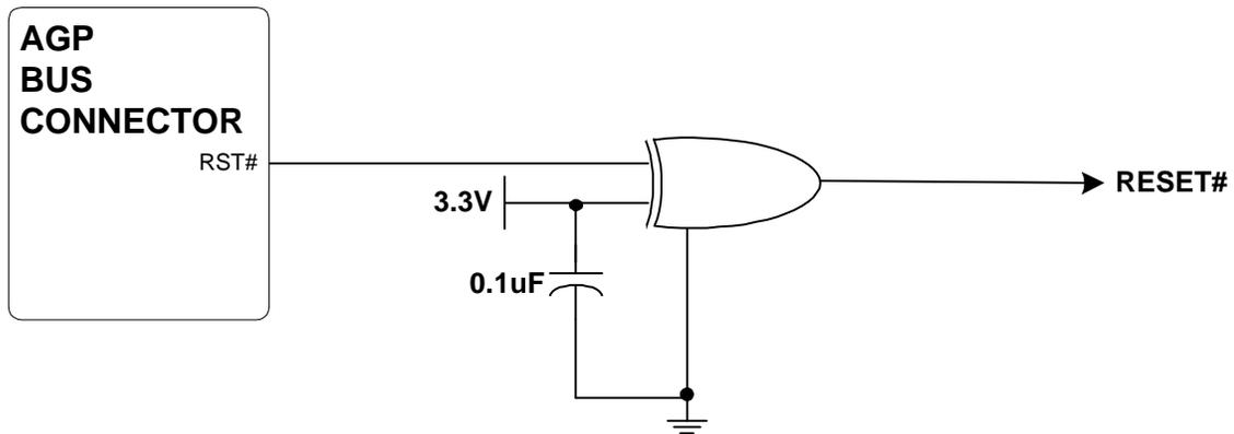
**Figure 7: RESET Buffer Circuit**
