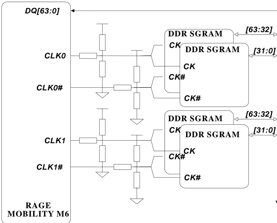
**Figure 17: Memory Clock: Termination and Distribution for the 64-Bit DDR**
