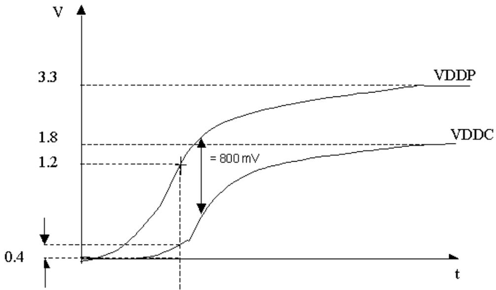
**Figure 4 Power sequence when VDDC derives from VDDR**
