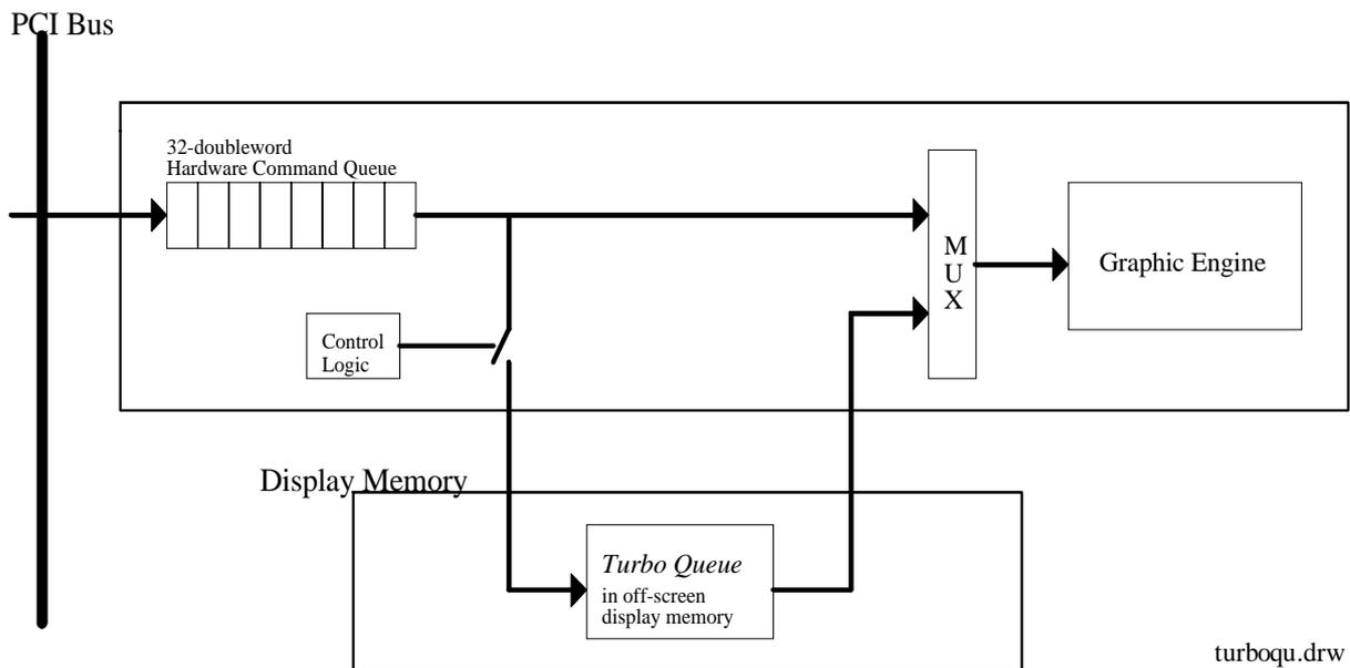
**Figure 3-33 Turbo Queue Architecture**
