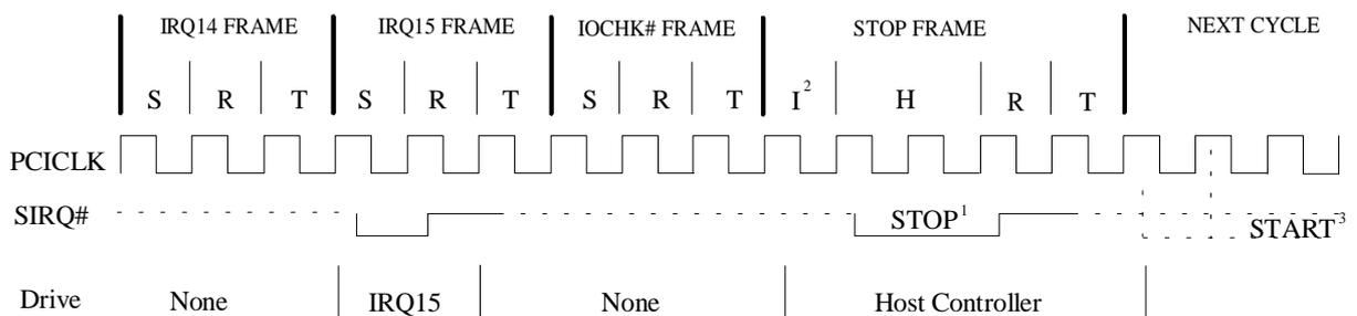
H=Host Control R=Recovery T=Turn-around S=Sample I=Idle
