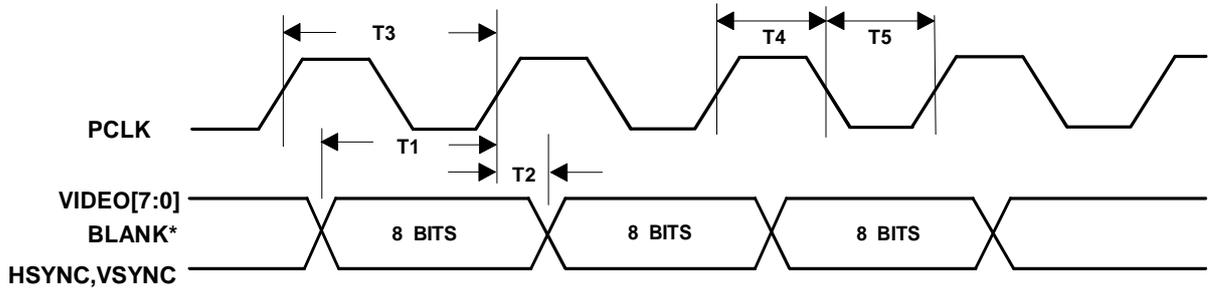
Figure 7-1 Video Timing 4, 8, 24 Bits/Pixel Modes
