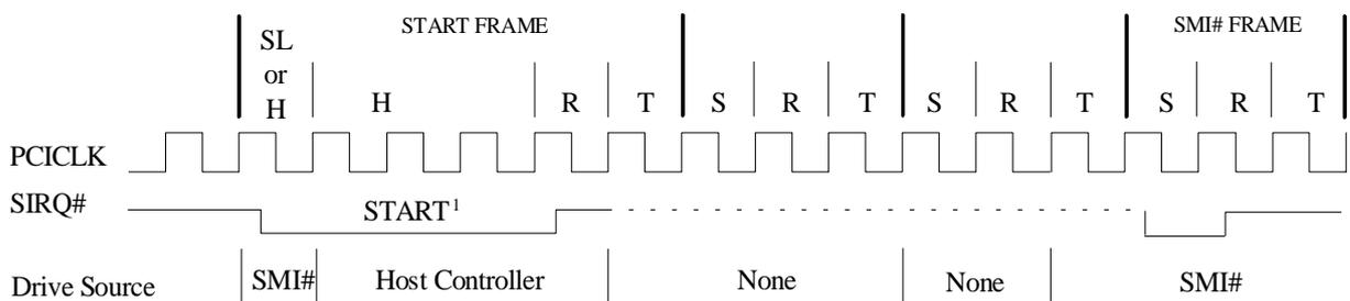
H=Host Control SL=Slave Control R=Recovery T=Turn-around S=Sample
