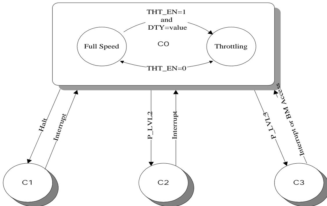
**Figure 3-17 Processor Power State Diagram**
